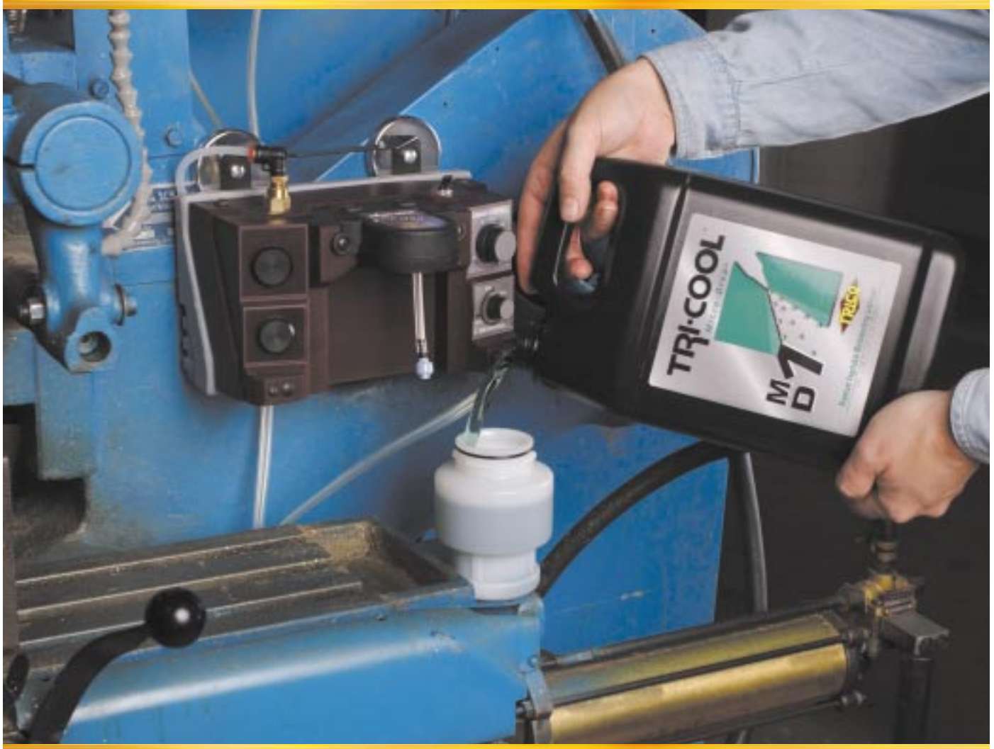
Micro-dispenser being filled with Tri-Cool MD-1 lubricant.
