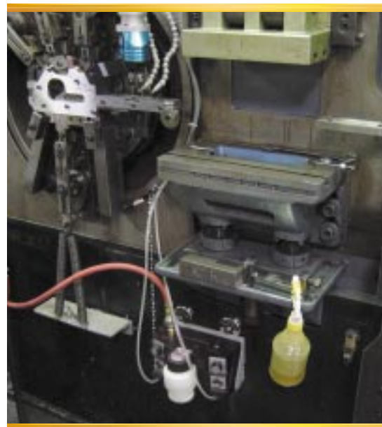
Minimum quantity lubrication used in a tapping workcenter.
